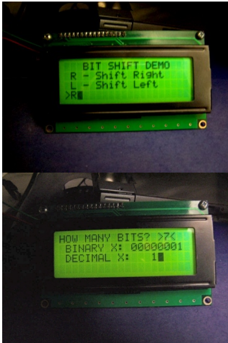
EXAMPLE 18 -- MENU-DRIVEN, SHIFT-RIGHT / SHIFT-LEFT DEMO: USES PS/2 KEYBOARD AND LCD PANEL
