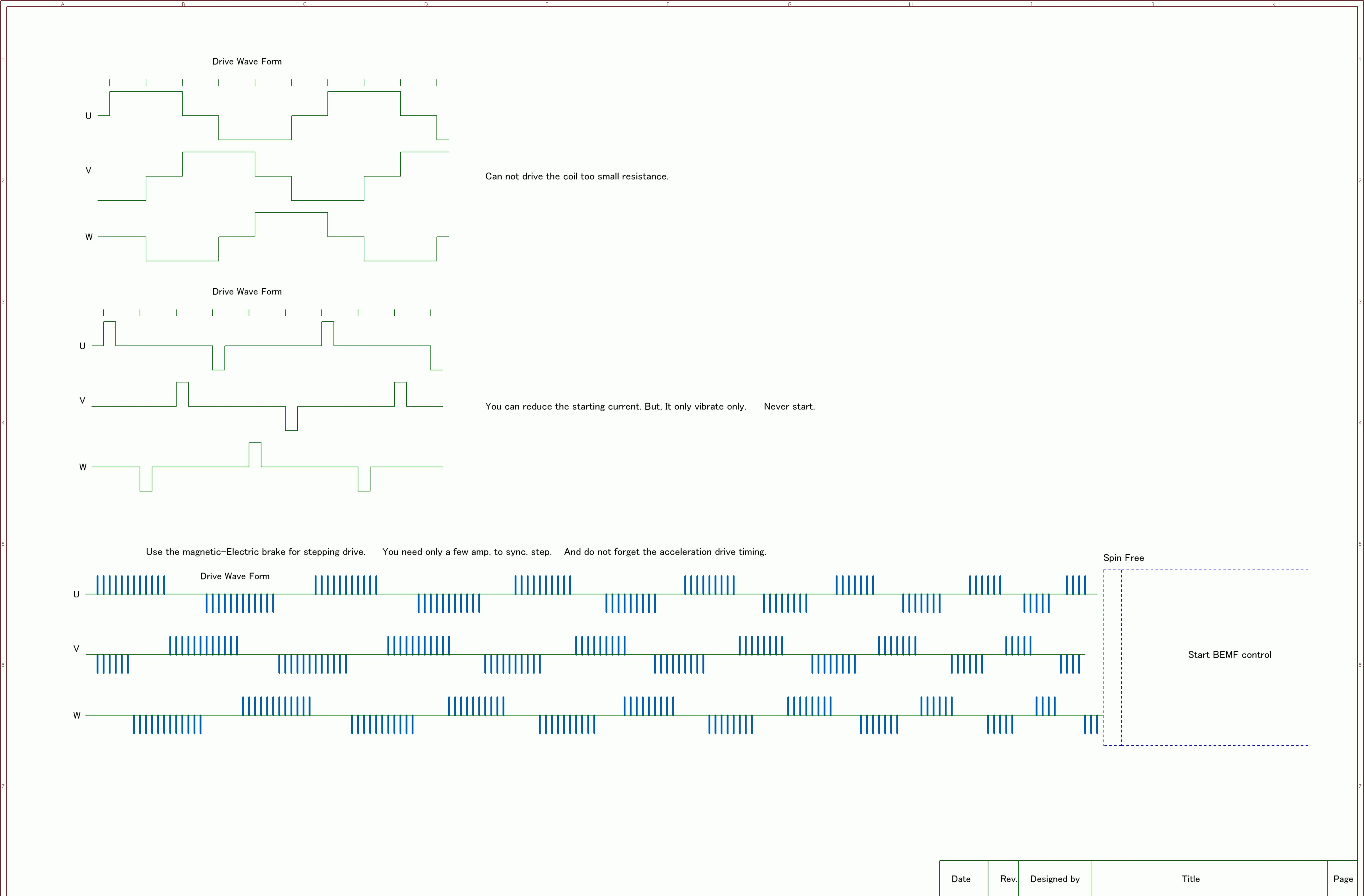
Takao Shimizu Sensor-less Brush-less Motor starting control image
