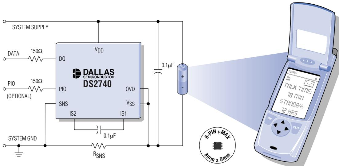
The DS2740's 15-bit current measurement has a resolution of 78 $\mu$ A and a 2.56A dynamic range when used with a 20m $\Omega$  sense resistor. An analog input filter extends this dynamic range for pulse-load applications. With a current ADC offset of less than 2 $\mu$ V and a gain error of less than 1%, the DS2740 provides a highly accurate report of remaining battery capacity.
