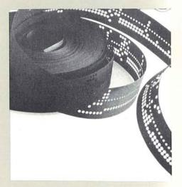
**Drill Tapes.** Automatic insertion equipment requires precise drill holes board-to-board. Drill tapes produced by the system provide consistently precise registration.
