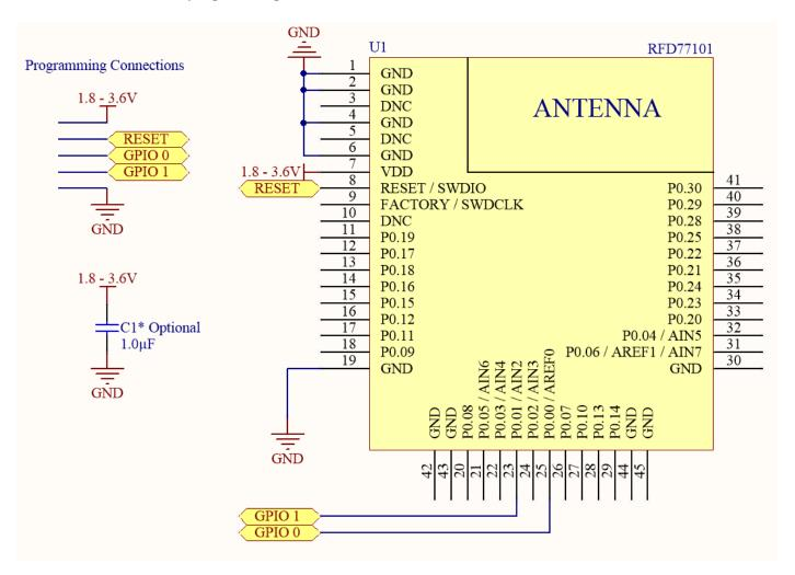
Note: A bypass capacitor C1 is recommended and should be placed close to pin 7.
