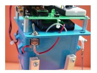
Here are the power switch and battery. The Battery is made of 5 NiMH AA tabbed cells soldered in series and taped. The super sophisticated battery hold down is by tie wraps. Yeah, I know, one is broken in the picture. It's fixed now.
