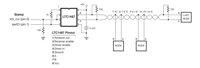
Figure 1. Networking demo setup.
