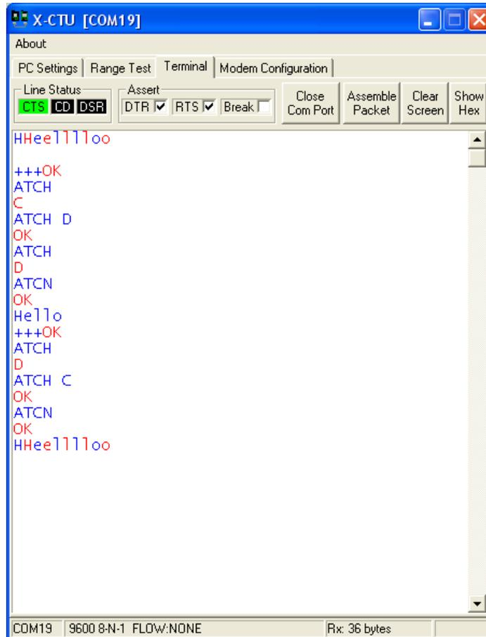
Figure 3-9: Using AT Command Mode in Terminal
